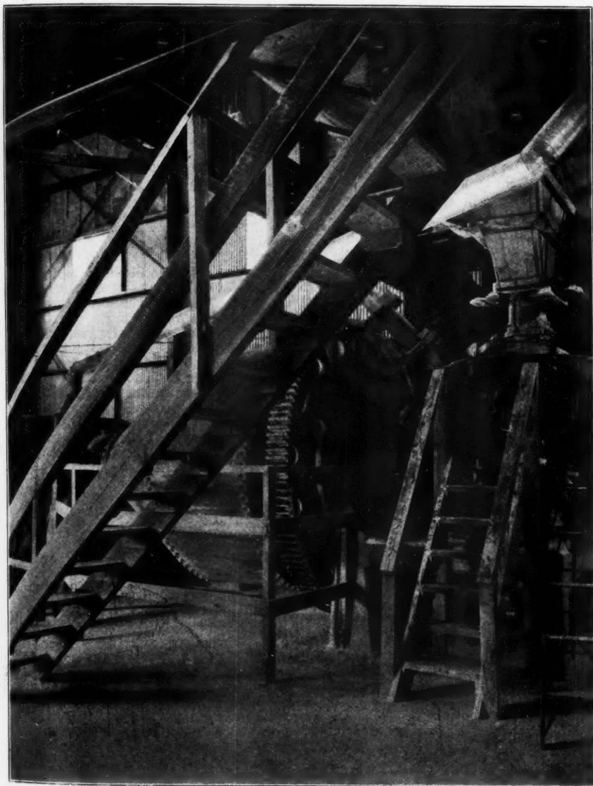
Interior View Showing Pebble Mill
